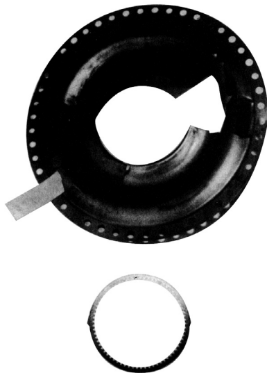
Outermost diaphragm of a coupling that failed due to overly-high misalignment. The rest of the coupling continued to operate for more than 10 million cycles
